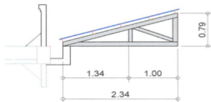
RAFTER DETAIL SCALE 1:50MTS
