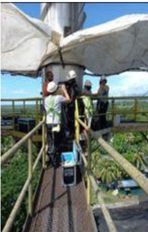
Particulate Matter Testing of Boiler Smokestacks
