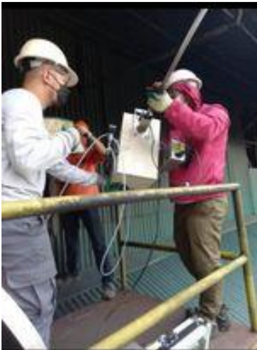
Nitrogen Oxides as \text{NO}_2 and Carbon Monoxide Testing of Generator Sets
